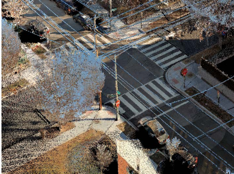
Figure 1. LiDAR Data at 4 th St NW and Decatur St NW
